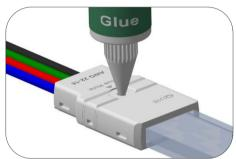
8. For waterproof treatment, align the injection hole of the connector with supplied silicone sealant, and inject until the silicone sealant slightly over flows from sides.
