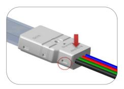
7. Once positioned correctly, Apply pressure until clipped down securely. Use of pliers is recommended at this stage.
