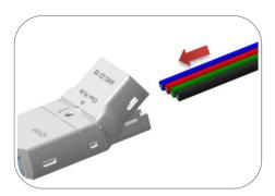
Cut the required wire length without stripping the wire insulation and insert it into the guided grooves.
