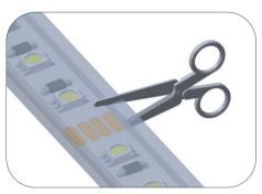
1. Cut strip light to the required length using the provided cut points on the tape.
