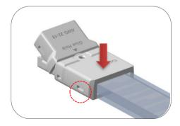
5. Once positioned, Apply pressure until clipped down securely. Use of pliers is recommended at this stage.
