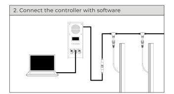
Using a network cable connect the the signal input port on the controller (DATA IN) with the device that contains the software.
