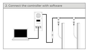
Using a network cable connect the the signal input port on the controller (DATA IN) with the device that contains the software.
