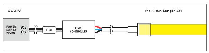
► This product must be installed by a suitably competent person. Check polarity (+/-) is correct before turning on. Incorrect polarity can cause damage to the product.
